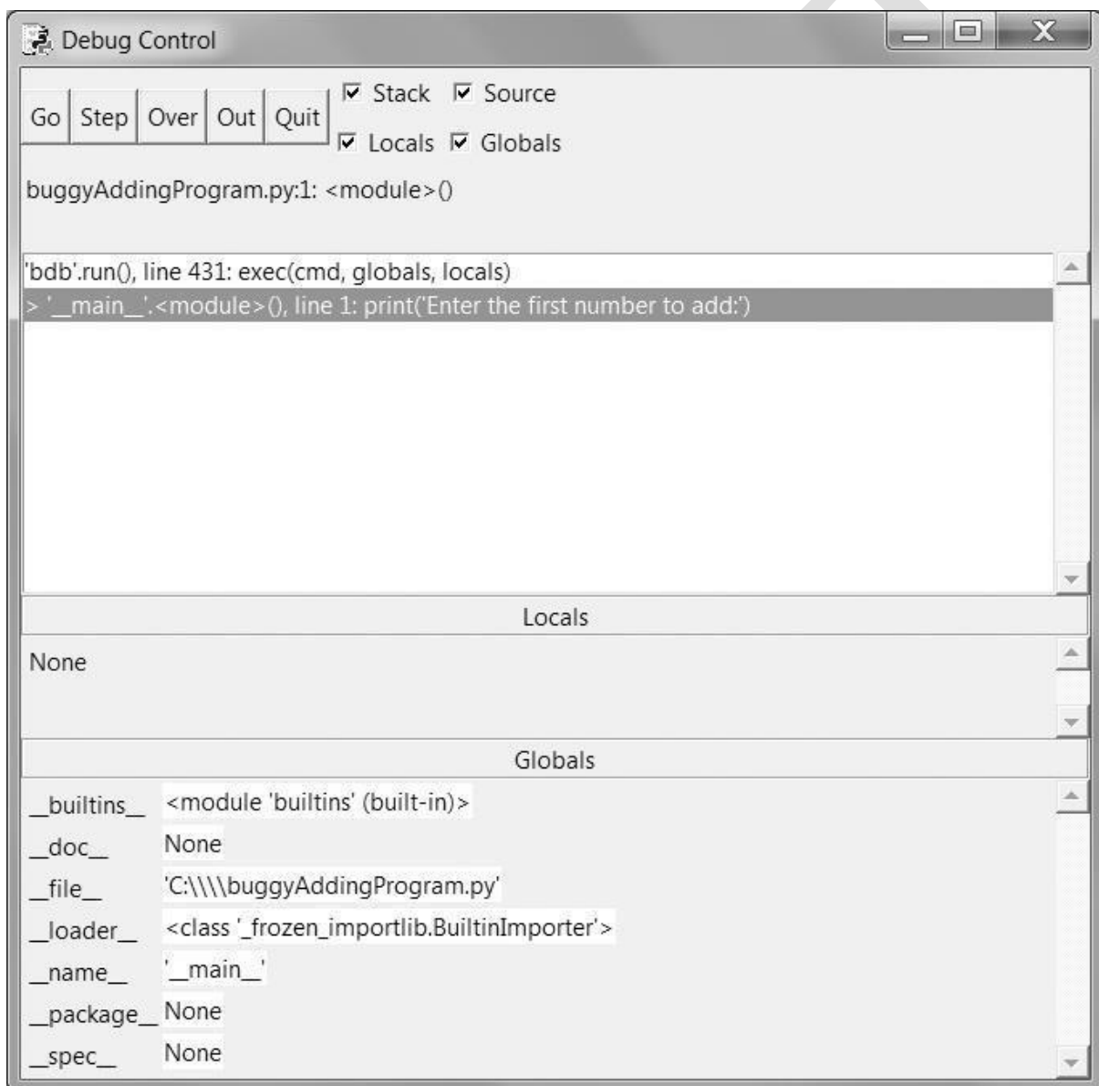
Figure The Debug Control window when the program first starts under the debugger
