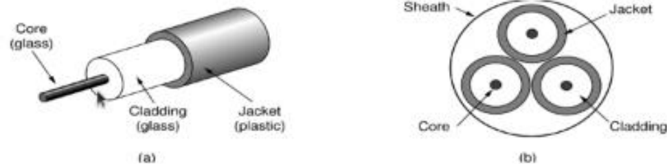
Fig. Views of a fiber cable
